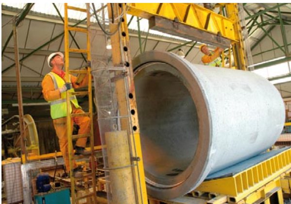
Testing a 1200 mm pipe for strength.
